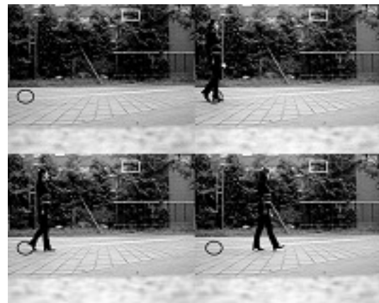
Fig. 7. Stationary pixel (white rectangle) and pixel that changes due to the object motion (black ellipse) in frame 1, frame 23, frame 33 and frame 50
