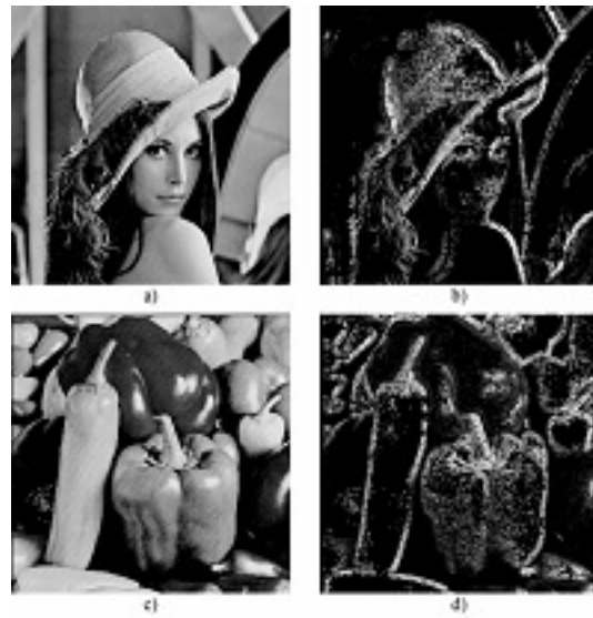
Fig. 2. a) Original image Lena, b) pixels of image Lena that are suitable for watermarking, c) original image Peppers, d) pixels of image Peppers that are suitable for watermarking
