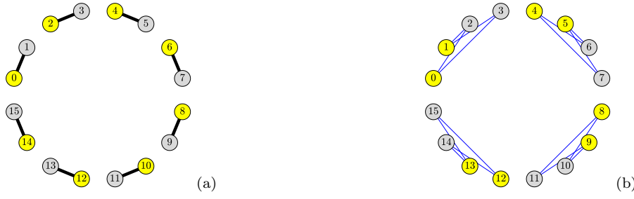
Fig. 33 Bipartite graph for the Haar wavelet transform with N = 16 vertices. (a) Vertices in yellow are used for the low-pass part of the signal and correspond to the set \mathcal{E} , while the vertices in gray belong to the set \mathcal{H} . This is the highest two-vertex resolution level for the Haar wavelet. (b) Graph for a four-vertex resolution level in the Haar wavelet.
